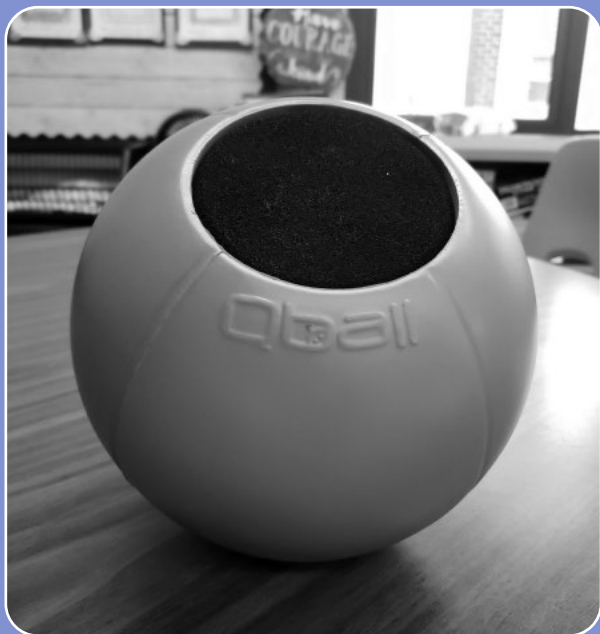
The Q-ball is a great tool for building confidence and increasing student participation in class. A microphone in the shape of a small ball, the Q-Ball is connected to the classroom's speaker system and is often passed around the classroom during instruction. Speaking into the Q-Ball allows students to have their voice more clearly heard.
